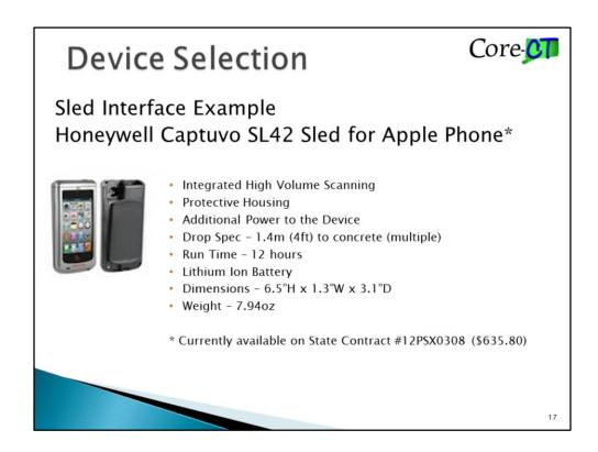
A sled allows a smartphone protection and integrated scanning capability. Sleds act as the scanner and the case (all in one). They also offer additional power capability. Typically the sled needs to be matched to the exact smartphone (just like a case for an IPhone 5 would not fit an IPhone 6).
